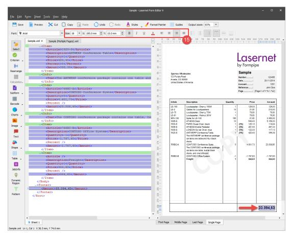
16. On the Developer toolbar, select the **Text** tool and insert the **Total** text. For the added text, set **Font size** to **18 pt**, the **X** position to **133 mm** and **Y** to **15 mm**. In the **Absolute** group box, select the **Last** and **Single** check boxes, set **Relative to** to **End of cond. area** (**Absolute**).
